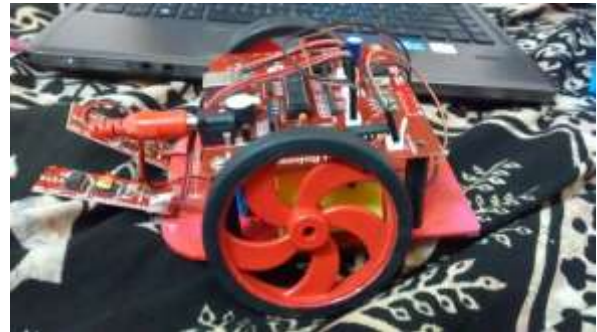
(Actual obstacle avoiding Robot after construction)
